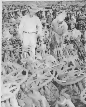
A big job of the Reclamation Yard is reclaiming valves, making them as good as new so they can be used again. Jacobo Cress (wearing hat), assistant reclamation sub-foreman, and Francis De Gale are seen among valves that will be reclaimed.
